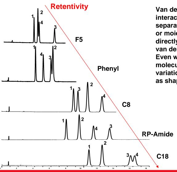
Van der Waals interactions are the main interaction responsible for the separation of hydrophobic molecules or moieties. Amylbenzene retention is directly related to the strength of the van der waals interactions of a phase. Even with strictly hydrocarbon molecules, there are selectivity variations based on such phenomena as shape selectivity.
